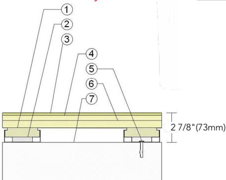
1. Steel Encased Plywood Sleeper
