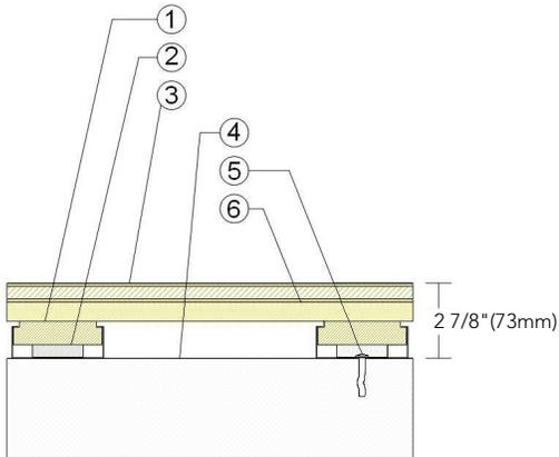
1. Steel Encased Plywood Sleeper
