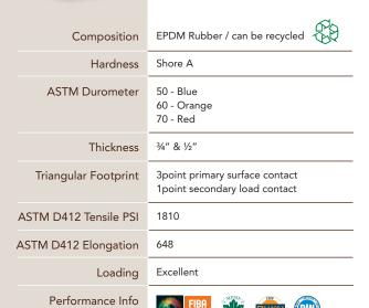
Tested to meet DIN 18032 Part II Tested to meet EN 14904 Tested to meet M.F.M.A.'s pur standards ASTM 2137 low temperature brittleness, 3 min @ -40 - pass ASTM D395 compression set, 22 hours @ 70c set % -20
